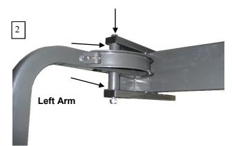
Insert Arm into position inside the Bearing Housing frame. Attach with M10 long bolts, washers and lock nuts. Do not over tighten—the Arms should pivot freely.
