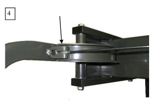
Attach cable to one of the Arm channels and thread the Idler Pulley on the cable before connecting to the other Arm.
