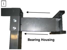
Remove the two long bolts at the top of the main frame. Position the Bearing Housing over the frame and replace the bolts with the two M12 long bolts, washers and lock nuts. Tighten firmly.
